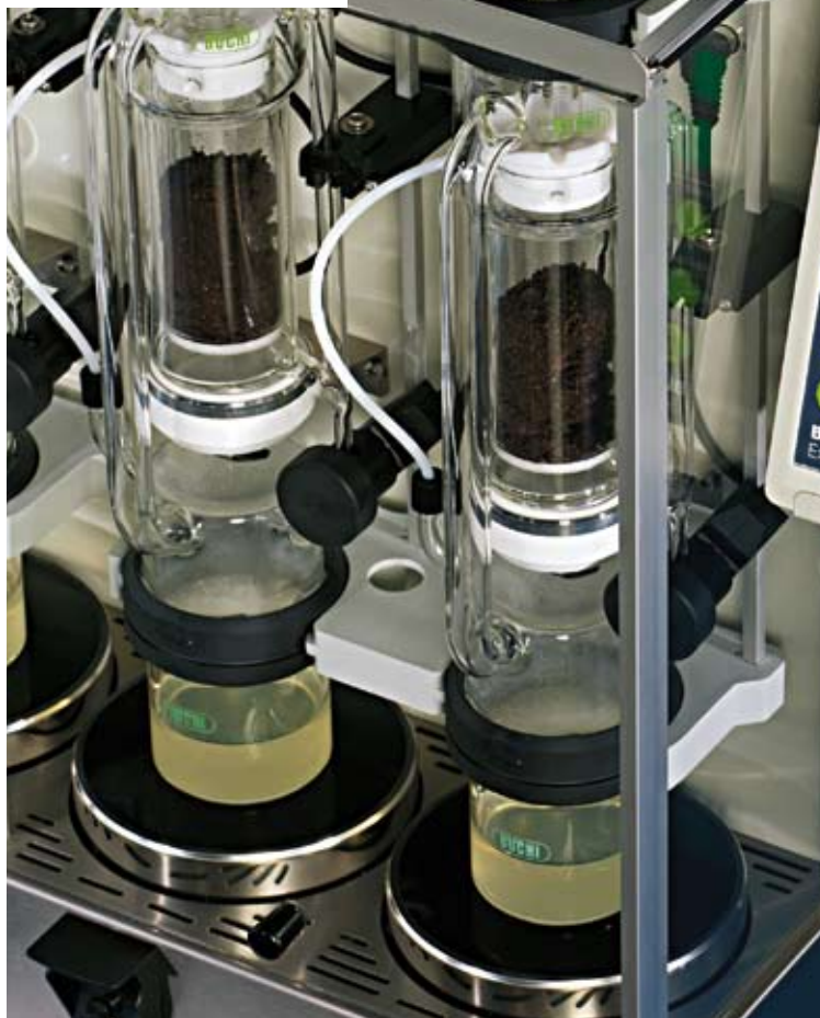
Extraction System B-811 Extracting PCDD/F from Soil and Grass Samples
